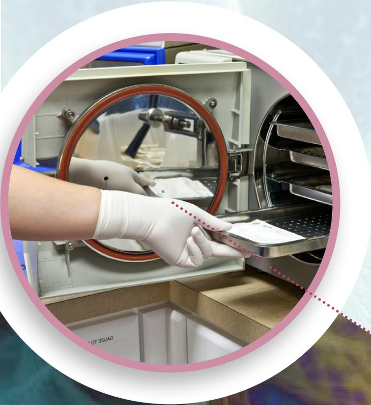
Spore testing or biological monitoring of sterilizers is required in many states and the Centers for Disease Control recommend that spore testing be performed on each sterilizer in your office every week.
